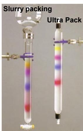
With slurry packing column (left-side of photo), the peak appears broad and tailing, indicating incomplete purification with poor purity and low recovery, and therefore low sample loading capacity.
