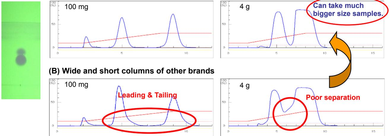
Yamazen columns are free of leading and tailing of peak. Compared to other brands of short columns, Yamazen columns can take much larger size samples.
