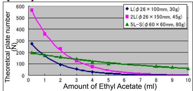
If the sample is dissolved in polar solvent like ethyl acetate, the performance of 5L-S Series columns remain nearly unaffected.
