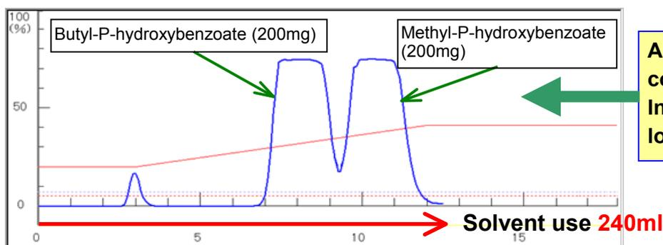
A pair of an Universal column L (40g) and an Inject column M for sample loading are used.
