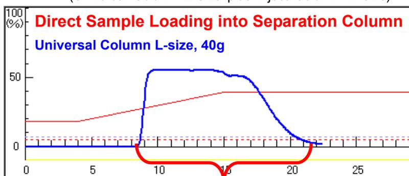
Two compounds eluted together, not separated by using DMSO to dissolve the sample.
