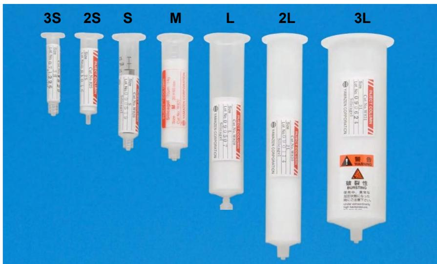
Inject columns are exclusively used for sample loading and are used with main separation columns such as Universal columns, Ultra Pack columns, etc.
