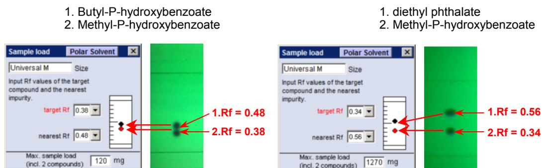
Our sample loading software has been designed to give the accurate number of maximum sample load for each column, assuring the resolution of  $R_s=1.0$ , based on  $\Delta R_f$  (distance between the target compound and its nearest impurity).
