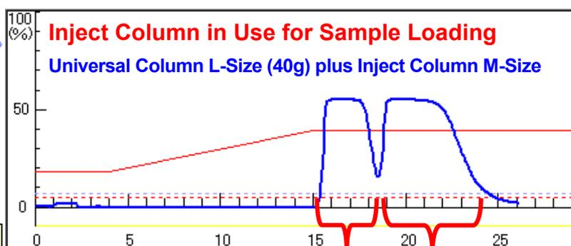
Two compounds were separated well with use of Inject column together with Universal column.
