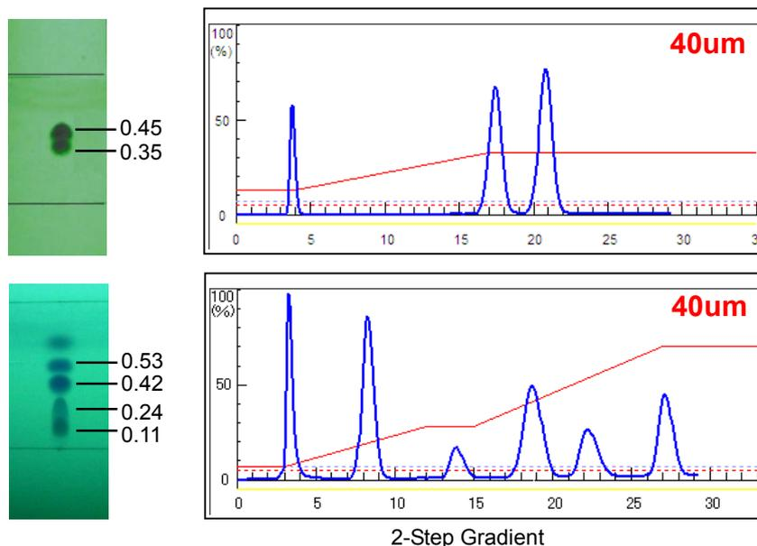
Universal columns are available in Normal Phase (Silica, Amino) and in Reverse Phase (ODS (C18)). Universal columns are available, packed with irregular silica gel of Pore Size 60 A, Particle Size 40-63 micron and also in Pore Size 60 A and Particle Size 25-40 micron (Premium).
