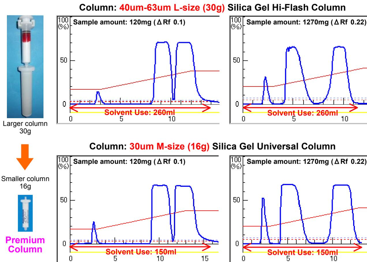
**Column Downsizing → Less Solvent Use → Save Laboratory Cost**
