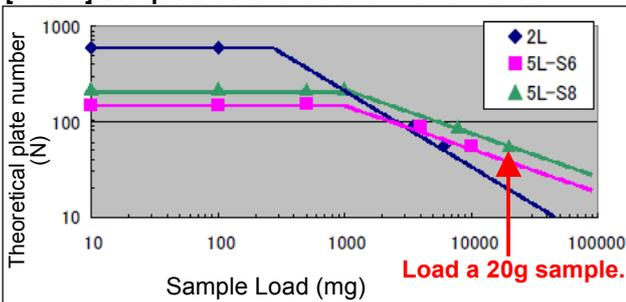
When loading samples in the gram scale, the 5L-S Series show higher theoretical plate numbers than the 2L.
